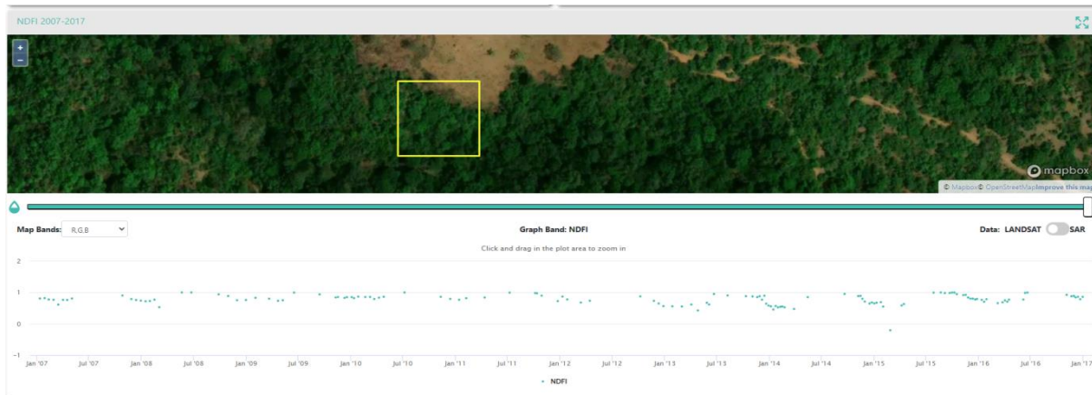
Figure 14 Collect Earth interface for data collection and Google Earth Engine platform for enabling time series imagery for sample plots using Landsat, MODIS and other available imageries.
